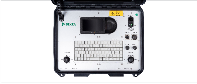
VT 334 FWSD CU open, control panel
