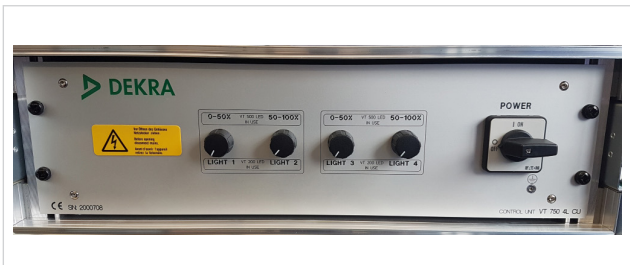
VT 750 4L CU Control unit to connect and to control 2x VT 500W R LED at the same time
